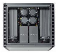
A large array of 32 high-current output devices drive the amplifier output stages reducing the load on individual components and are supported from 188,000uF of patented bulk storage capacitors delivering huge continuous power for fast but smooth, accurate audio with great rhythm and timing, even under extreme loading conditions.
